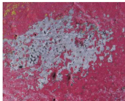
Figures 10.69 (above left) and 10.70 (above right): Details of cleaning trial 104-T.13 in normal (left) and raking light (right). Removal of the graffiti paint is limited and results are inhomogeneous. Furthermore, the original paint layer has been visibly damaged and worn away in areas. Photo: Courtauld Institute CWPD 2007
