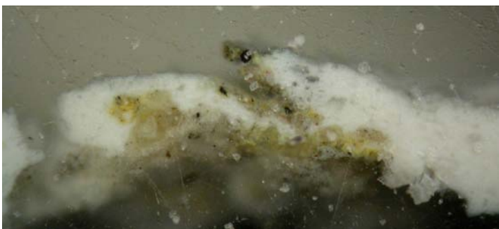
Figures 10.76 (above left) and 10.77 (above right): X-section 3895, 200x; under normal (left) and UV (right) lights. The surface of the cleaned paint layer appears rougher than the control sample and no evidence of the coating remains after cleaning. Although the sample is heavily fractured, this is likely due to sampling procedure rather than specifically to damage caused during cleaning. Photomicrograph: Courtauld Institute CWPD 2007
