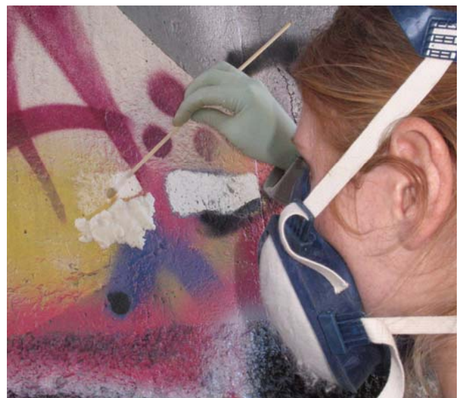
Figure 10.54: The final cleaning trial (104-T.21) was carried out with the application of a solvent mixture in Arbocel B800. The Arbocel was applied to the mural surface and could be removed section by section. In this way it was possible to avoid evaporation of the solvent from the graffiti paint before the added materials were adequately removed by swabbing with free solvent. Photo: Courtauld Institute CWPD 2007
