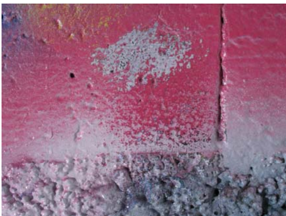
Figure 10.68 (above): Results of cleaning trial 104-T.13. The results are extremely poor in comparison to the results achieved with the developed system in cleaning trial 104-T.21. Photo: Courtauld Institute CWPD 2007
