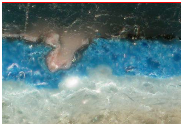
Figure 10.41: The original paint layer is shown at high magnification (500x) with coating present. Photomicrograph: Courtauld Institute CWPD 2007
