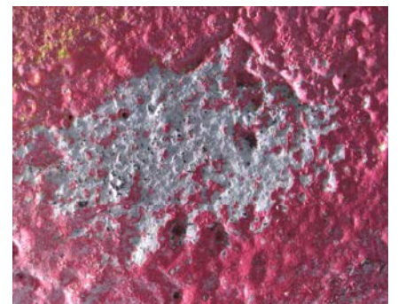
Figures 10.69 (above left) and 10.70 (above right): Details of cleaning trial 104-T.13 in normal (left) and raking light (right). Removal of the graffiti paint is limited and results are inhomogeneous. Furthermore, the original paint layer has been visibly damaged and worn away in areas. Photo: Courtauld Institute CWPD 2007
