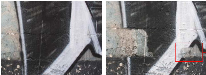
Figures 10.18 (above left) and 10.19 (above right): Site of trial 102-T.19; pre-cleaning (left) and post-cleaning (right). Photo: Courtauld Institute CWPD 2007
