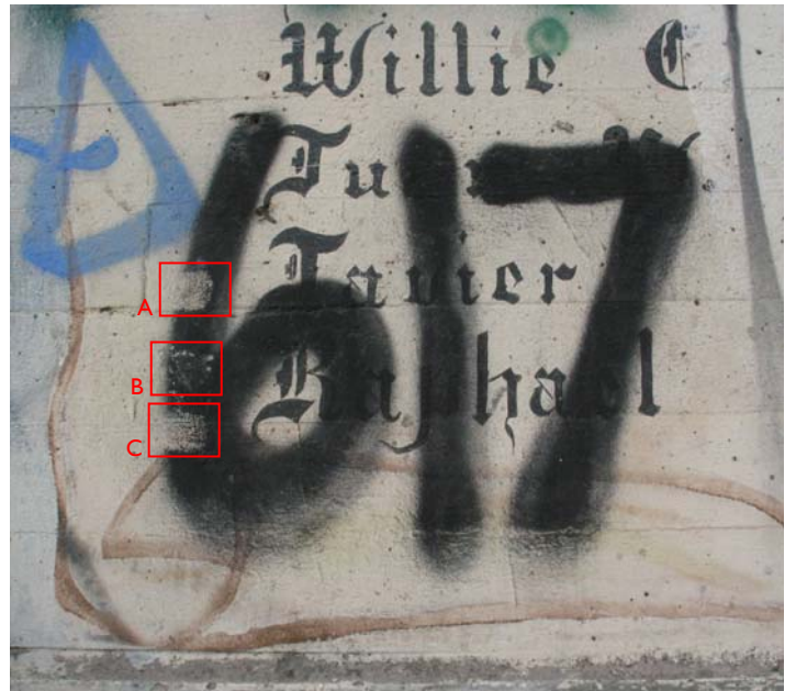
Figure 10.133: Site of final cleaning trials on the more soluble aerosol graffiti paint. Photo: Courtauld Institute CWPD 2007
