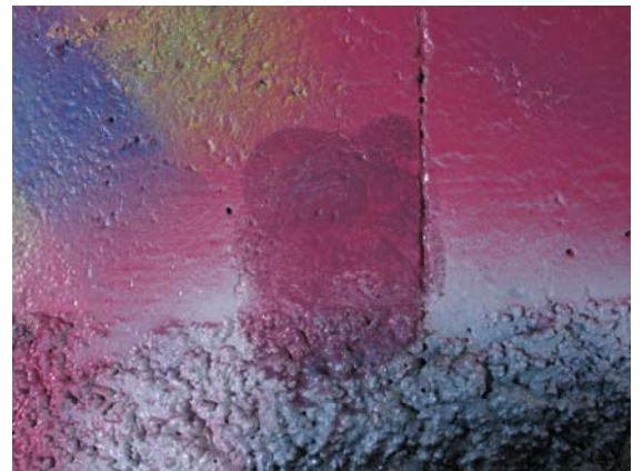
Figure 10.67 (above right): During trial 104-T.13 in which the proprietary graffiti-removal product, Graffiti Gold Remover™, was used for cleaning. Photo: Courtauld Institute CWPD 2007
