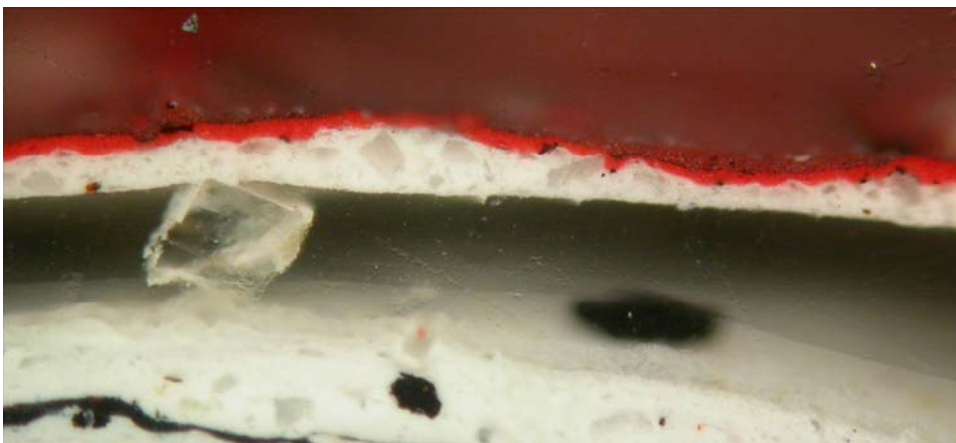
Figure 10.110: X-section 4086, photographed at 200x. Based on its location, the cleaned sample should have a thin black paint layer across its surface. Mobilization of this layer was observed during cleaning however and only slight traces of the layer are visible in the cross-section taken from this area. Photomicrograph: Courtauld Institute CWPDP 2007
